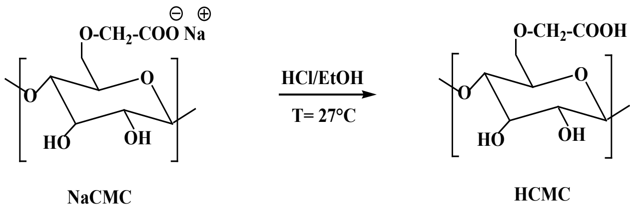
Fig. 1. Acidification reaction of NaCMC using ethanol.
